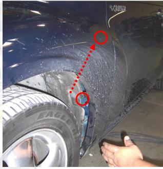
Remove all the 10mm bolts from the top of the fender. You will need to use a wrench to remove the last 10mm bolt located by the windshield pillar.
