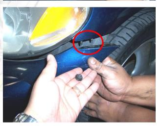
Remove (1) 10mm bolt from the front of the bumper, pull back on the bumper to gain access to (1) 10mm bolt that secures the fender to the body.
