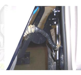
**11)** Cut the inner lip of your fender to make room for the new Vertical Doors hinge. Note: After you have cut the fender use a sander or grinder and make sure the surface is completely flat.
