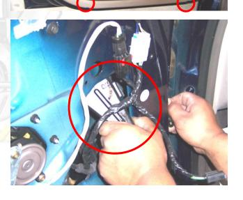
**4)** Modify the factory wire boot: Use the fork to help you pull the factory wire boot off the car, cut the wire shrink wrap so that the wires come loose, this will let you pull on the wires to gain more wire slack. Also cut the factory wire boot in half.
